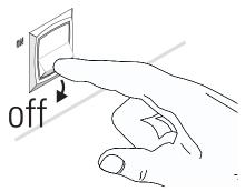
To turn the amplifier 'off', push in on the bottom portion of the rocker switch firmly. It should move inward and snap into the 'off' position. After switching off, the power LED should extinguish.
